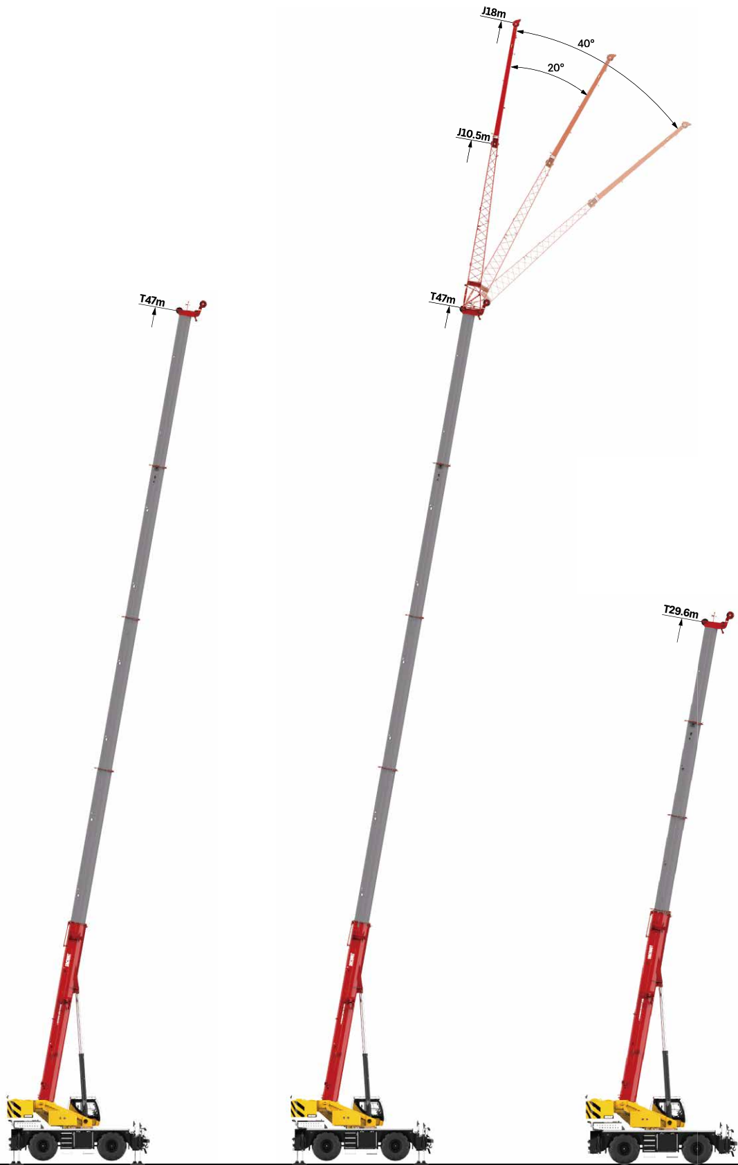
Telescopic boom on outriggers 主臂、支腿吊载
