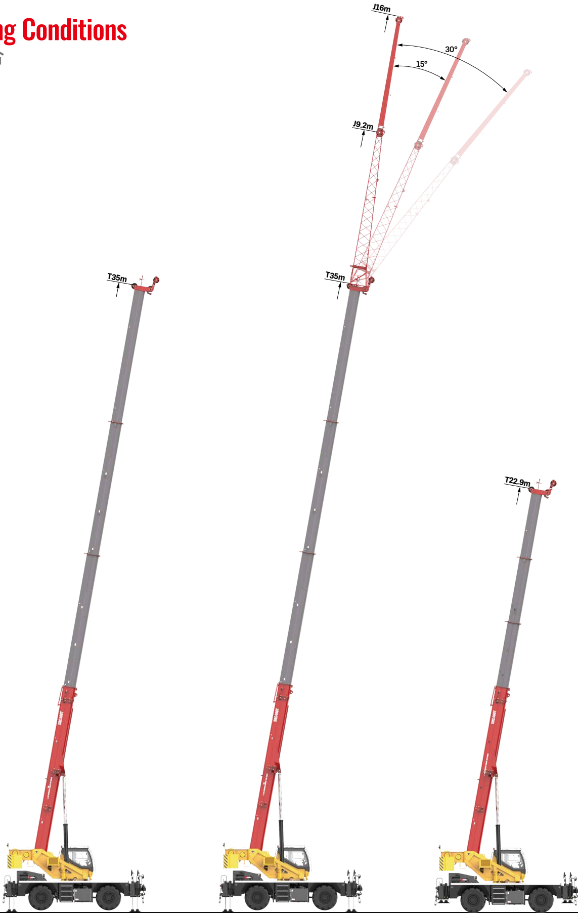
Telescopic boom on outriggers 主臂、支腿吊载
