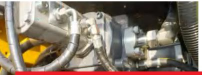
**REXROTH HYDRAULIC SYSTEM** Load-sensitive hydraulic system Adjustable pressure and flow of the AUX pipelines. Variety of accessories can be used.
